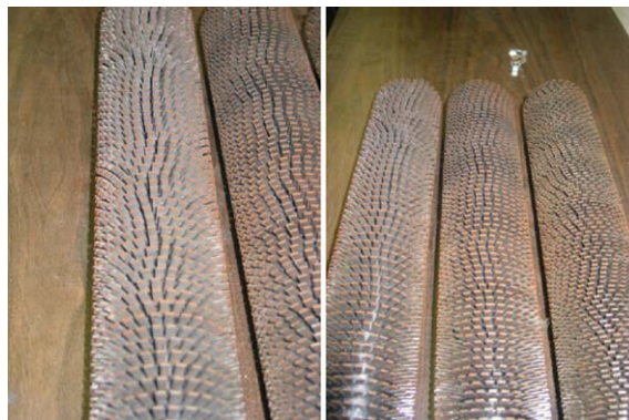
Fig. 14. Photographs of the finned tubes showing the wavy pattern.
